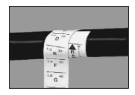
4.02 Puncture and cut through range letter on front side of each seal.
