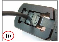
Place jack into crimper tool and crimp
