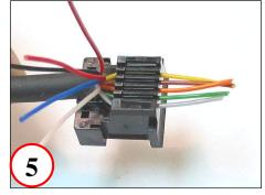
Place lower row conductors into load bar
