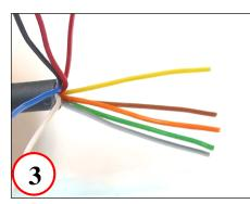
Align lower row conductors, fold upper conductors out of way
