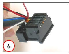
Trim lower row flush with front of load bar
