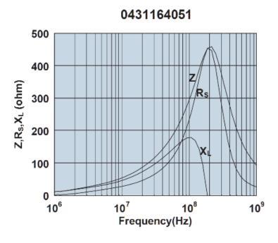
Impedance, reactance, and resistance vs. frequency.
