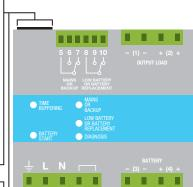
Jumper present: life test enabled. Jumper present: fast test enabled. Jumper present: fast recovery charge enabled only for size 3. Possibility to recharge the battery also when the voltage is close to zero with the maximum power of the device.
