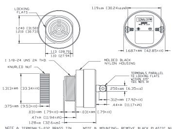
NOTE A: TERMINALS-032 BRASS TIN PLATED, TAPPED FOR #6-32 SCREW. TWO #6-32 NICKEL PLATED BRASS SCREWS INCLUBED, WILL ACCEPT 1/4\* QUICK CONNECT.
