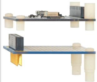
For the overlapping configuration, install the standoffs into all four mounting holes of the P8X32A QuickStart and tighten each into a nut.
