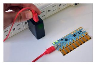
Finally, USB phone charger battery packs work as a handy portable power supply! Make sure your charger battery pack has an on/off switch so that you can keep the power supply on. The Chibi Chip runs on low power so the battery pack may automatically turn off by itself.
