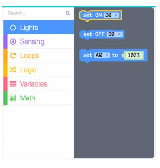
Link the blocks together to blink the LED like so.
