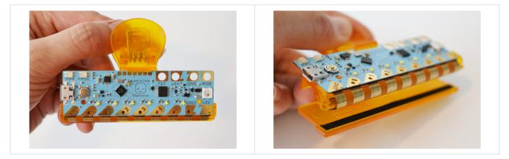
Try creating a simple circuit with one LED and traces that align to the Chibi Chip and clip's tabs.
