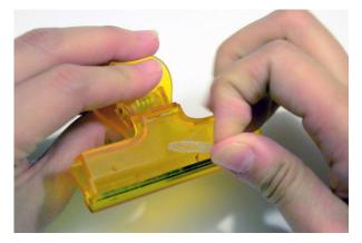
Flip the clip over so that the flat side showing "Chibitronics" faces up and open the clip.
