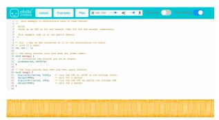
That means the code is being uploaded! When the code is done uploading, the red PROG light on your board will turn back to green to let you know that programming is done successfully. Now you should see your LED blink on the defined pin. Congrats! You've uploaded your code. Your Chibi Chip should now have a light blinking!
