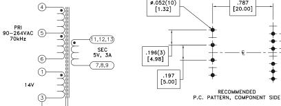
Application of the transformer allows for the leadwires between terminals 7&8&9 and 11&12&13 to solder bridge.
