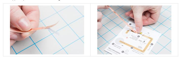
This template includes a few turns - to keep a solid connection of copper around corners, we'll be using a folding technique to press the tape into shape. Start by sticking the copper tape down until you reach the corner, then fold the tape backward on itself. Use a fingernail or pen to give it a good crease at the edge.
