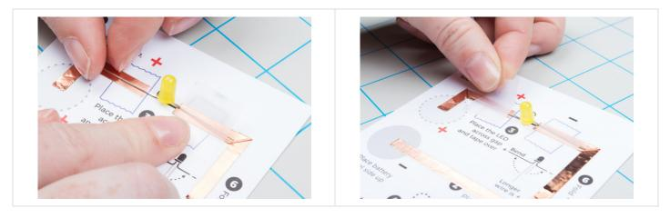
The connection between the LED and copper tape should look like the image below.
