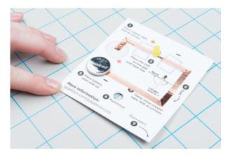
Carefully fold along the dotted line so that the copper tape inside the + circle rests on top of your battery, making a connection. You should see your LED light up once the copper tape touches the battery. Flip your project over and push the LED through the hole you punched to see it shine through the design.
