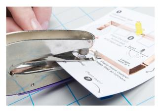
Depending on how centered you placed the LED over the gap in the copper tape, you may need to slide or slightly move it. Simply peel up the clear tape and adjust to center the LED in the hole. Then secure with some new tape. Fold the card over for a preview of where the LED will shine through on the template's design.
