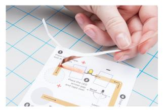
Then carefully move the tape down around the corner - you should see the fold forming - and press down flat against the paper. The neatness of the fold doesn't matter that much, it will be covered by your pop up in the end.
