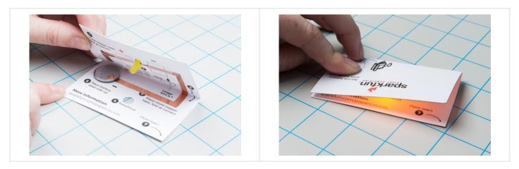
Secure the battery in the project using a binder clip. If you don't have a binder clip, a large paper clip can also work.
