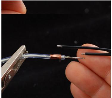
Next get your wire ready, ours come precut and tinned. If not, cut so that one side is about 1/2" longer than the other tin the ends. EL is AC-powered so you dont have to worry about 'polarity'.
