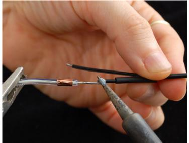
Pull the wire apart so that you can slip the heat shrink on and have 1/4" or more of clearance from the end of the wire, otherwise the soldering iron will prematurely shrink it. Solder the wire to the middle conductor.
