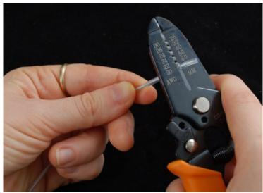
Next, we'll need to remove the outer coating. This is the hardest part of the process so don't be disappointed if it takes a few tries to get it right! Use the 20 AWG or 18 AWG slot and strip off the PVC coating about 1/2" (1 cm) away from the end.
