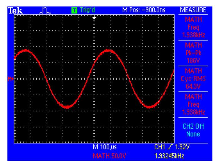
If you are comfortable using tools want to optimize your driver and wire, you can do so by 'modeling' your EL wire with a capacitor and resistor and plugging that in, then measuring the frequency across the RC with a multimeter or scope, just watch out you don't zap yourself!
