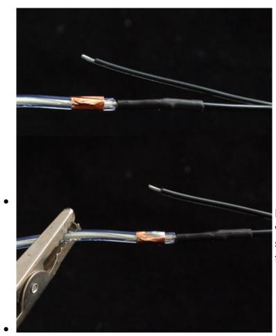
Now we can revisit the corona wires. Using the tip of the soldering iron, heat up the copper tape and melt a little solder on.
