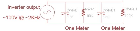
Of course, we can simplify by calculating the new capacitance and reistance. Remember that capacitance *increases* in parallel and resistance *decreases*.
