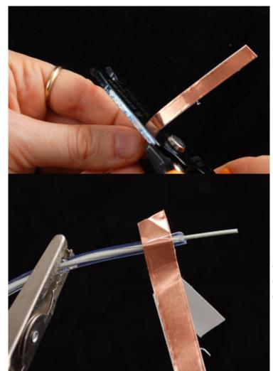
Next, cut a 1" or so piece of 1/4" copper tape. Dont use scissors to cut copper tape, use wire cutters!
