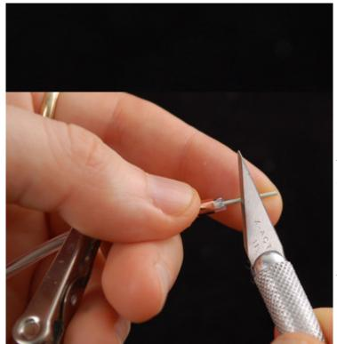
Now that the corona wires are tucked away safely, we can work on soldering to the middle wire. First we must remove the phosphor, by scraping it off. Some people use a lighter to burn it off but we like to just scrape it with a razor. Either way, remove some of it.
