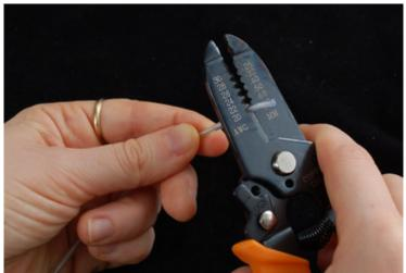
If you arent succeeding at getting the PVC off without damaging the wires, you can try not-quiteclosing the cutters all the way (the image below is an exaggeration of how much to close it) and giving it a good yank.
