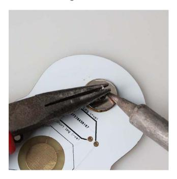
Next remove the iron while still holding in place with the pliers. This will stay very hot for a while so be careful!
