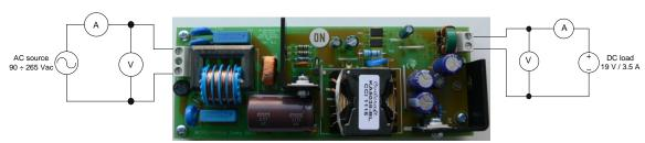
**Figure 1: Test Setup**
