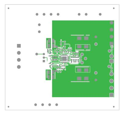
Figure 17. TPS40322EVM-074 Bottom Copper (bottom view)
