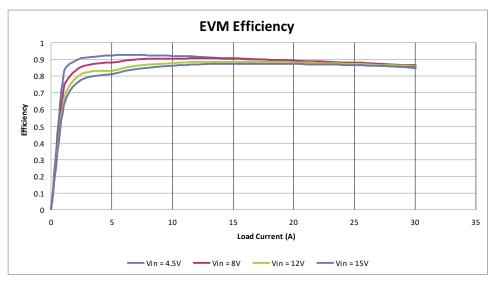
Figure 4. TPS40322EVM-074EVM Efficiency, (data measured from TP1 to TP3)
