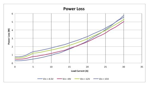
Figure 5. TPS40322EVM-074 Power Stage Power Loss, (data measured from TP25 and TP27 to TP24 and TP26)
