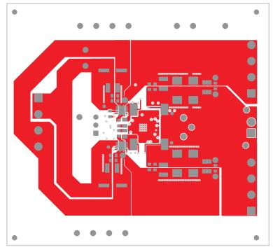
Figure 16. TPS40322EVM-074 Top Copper (top view)
