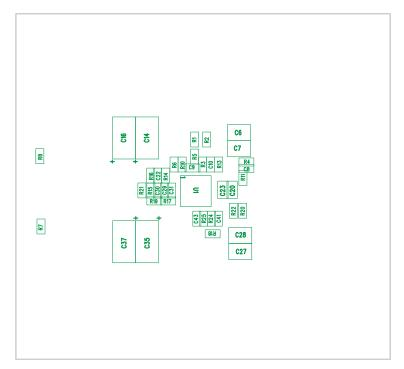
Figure 15. TPS40322EVM-074 Bottom Assembly Drawing (bottom view)
