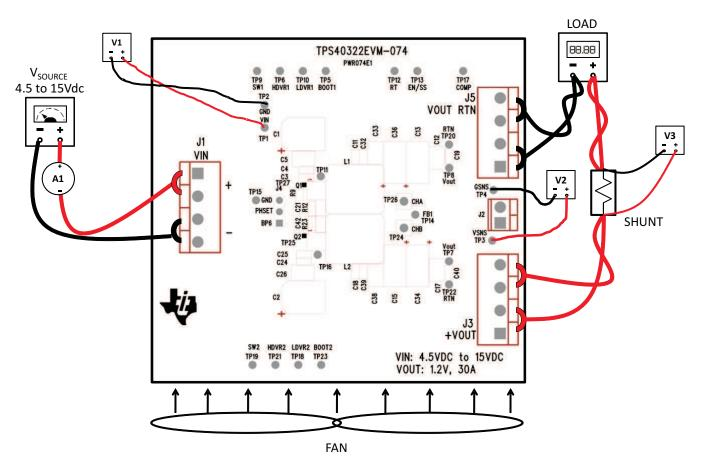
Figure 2. TPS40322EVM-074 Recommended Test Setup
