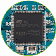
Figure 3-1: STM32F407ZG ARM® Cortex™-M4 Microcontroller
