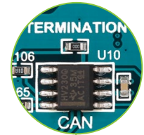
Figure 16-2: CAN transceiver with Node TERMINATION jumper
