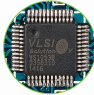
Figure 8-1: On-board VS1053 MP3 codec
