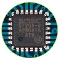
Figure 15-1: Ethernet transceiver module [LAN8720A]
