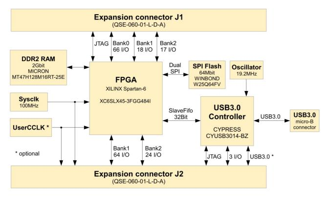
Figure 3: FPGA – USB3 board functional Diagram
