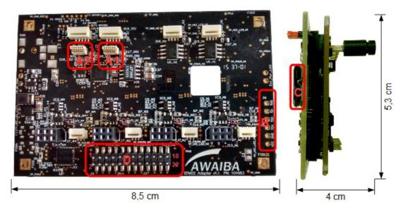
Figure 2: NanEye GS interface board
