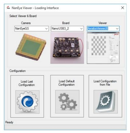
Figure 5: Starting the Viewer with the sensor connected on the J8 connector
