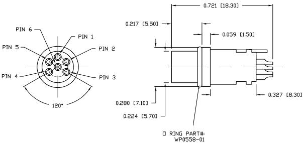
NΠΤF: MATERIAL HOUSING: PBT UL94V-0, BLACK CONTACT: **BRASS** NUT: **BRASS** GROUND: **BRASS** □-RING: NBR, BLACK **FINISH** GOLD PLATED CONTACT: □VER 504" NICKEL NUT: NICKEL PLATED GROUND: BRIGHT TIN (60 u") **ELECTRICAL** RATED CURRENT: ЗА RATED VOLTAGE: 125V INSULATION RESISTANCE: 1000 MOhms MIN. CONTACT RESISTANCE: 10 mOhms MAX. WATER PROOF: IP67 **ENVIRONMENT** OPERATION TEMPERATURE: -40°C TO +85°C MAX MATING TORQUE: 4-5 in lbs 854-006-203RLSY 1 = GOLD FLASH4 = 10u'' GDLD
