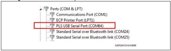
15. The COM port is configured and available to be used for serial communication with the PC.
