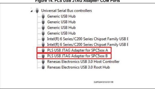
Figure 14. PLS USB JTAG Adapter- COM Ports
