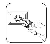
AC Input Connection: Insert L6-30P twist-lock plug into compatible L6-30R utility, generator or UPS outlet.
