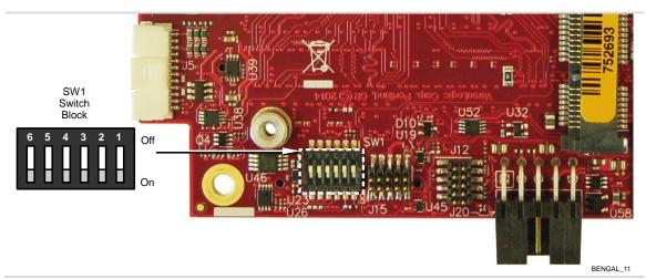
Figure 11. Location of SW1 Configuration Switch Block
