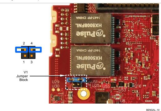
Figure 10. As-Shipped Jumper Settings
