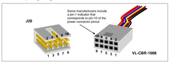
Figure 12. J20 and VL-CBR-1008 Pin Numbering
