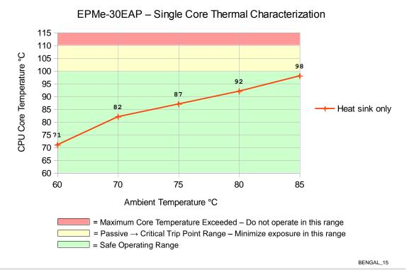
Figure 18. EPMe-30EAP CPU Core Temperature Relative to Ambient Temperature
