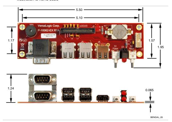
Figure 5. VL-CBR-5015 Dimensions and Mounting Holes
