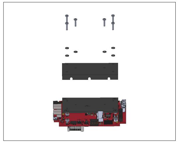
Figure 23. Installing the Heat Pipe Block
