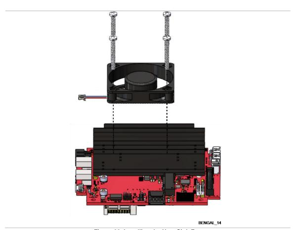
Figure 22. Installing the Heat Sink Fan
