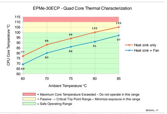
Figure 20. EPMe-30ECP CPU Core Temperature Relative to Ambient Temperature
