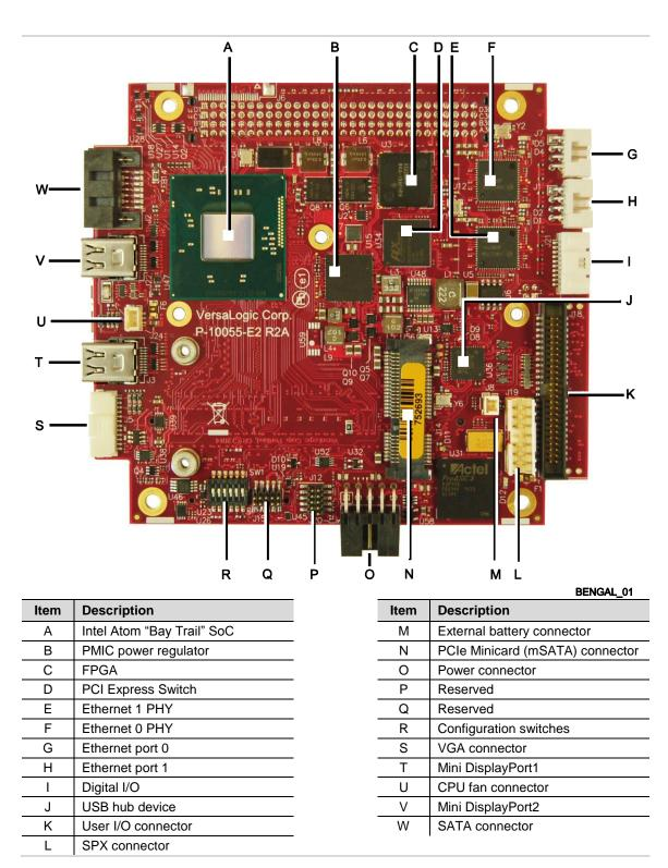
Figure 1. Major Components and Connectors (Top Side)
