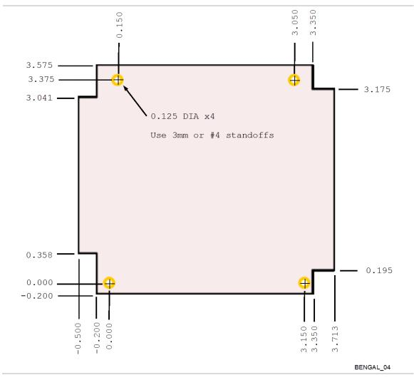
Figure 4. Bengal Dimensions and Mounting Holes
