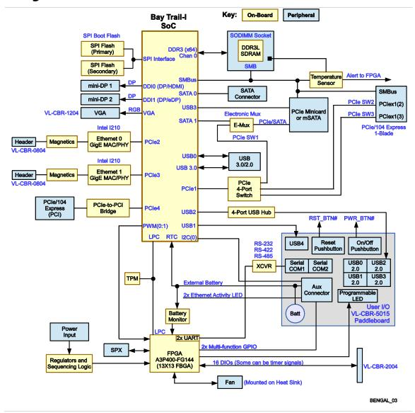
Figure 3. Bengal Board Block Diagram
