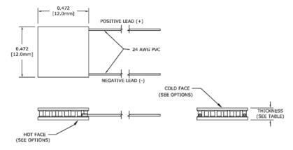
Ceramic Material: Alumina (AI<sub>2</sub>O<sub>3</sub>)
