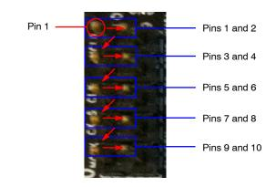
Figure 6. Pin Locations and Assignments of Grouped Jumpers. Pin 1 is Located at the Top-Left Corner and Increases in a Zigzag Fashion Shown in the Picture
