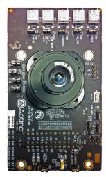
Figure 1. MT9M031 Evaluation Board
