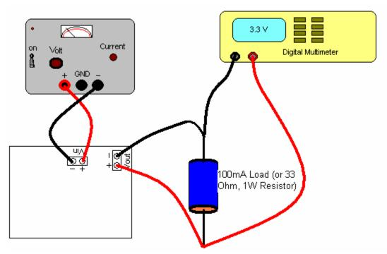
Figure 1: Test Procedure for MC34063
