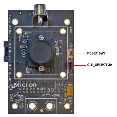
Figure 3. Top View of Evaluation Board – Jumpers
