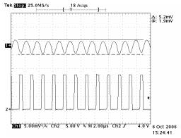
12Vin Output Ripple: CH1: Vou⊤. CH2: Switch Node taken at 0A Out.
