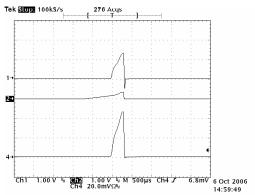
Short Circuit Protection: CH1:Vout. CH2:Sstart. CH4:Iout(10A/div).
