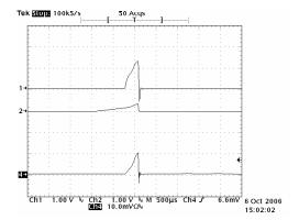
Short Circuit Protection: CH1:Vout. CH2: Sstart. CH4:Input Current (5A/div).
