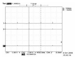
Short Circuit Protection: CH1:Vouτ. CH2:Sstart. CH4: Input Current (5A/div). 104ms restart rate shown.
