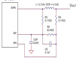
Over-current detection circuit for Imax > 60mV/DCR
