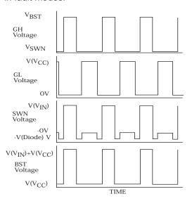
The second feature is a 100% duty cycle timeout that ensures synchronized refreshing of the BST capacitor at very high duty ratios. In the event that the high side NFET is on for 20 continuous clock cycles, a reset is given to the PWM flip flop half way through the 21st cycle. This forces GL to rise for the cycle, in turn refreshing the BST capacitor. The boost capacitor is used to generate a high voltage drive supply for the high side switch, which is Vcc above V<sub>IN</sub>.
