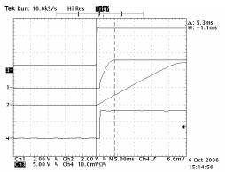
Start-up in to 3A Load: CH1:Vout. CH2:SS. CH3:Vin. CH4: lout (2A/div).
