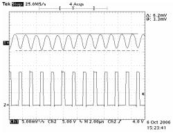
12Vin Output Ripple: CH1:Vout. CH2: Switch Node taken at 3A Out.
