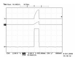
Current Limit: CH1: Vouт. CH2:SoftStart. CH4 louт (2A/div). Current is reaching approximtely 6A before a shutdown & restart
