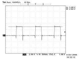
Operation from exernal bias: CH2: Switchnode @ 3VIN, IOUT = 3A.
