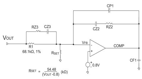
Type III Error Amplifier Compensation Circuit
