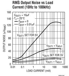
10Hz to 100kHz Output Noise  $C_{BYP} = OpF$
