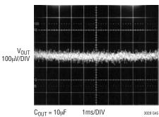
$C_{OUT}$  =  $10\mu F$  $I_L$  = FULL LOAD  $V_{OUT}$  SET FOR 5V
