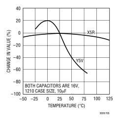
Figure 5. Ceramic Capacitor Temperature Characteristics
