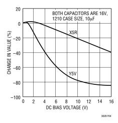
Figure 4. Ceramic Capacitor DC Bias Characteristics
