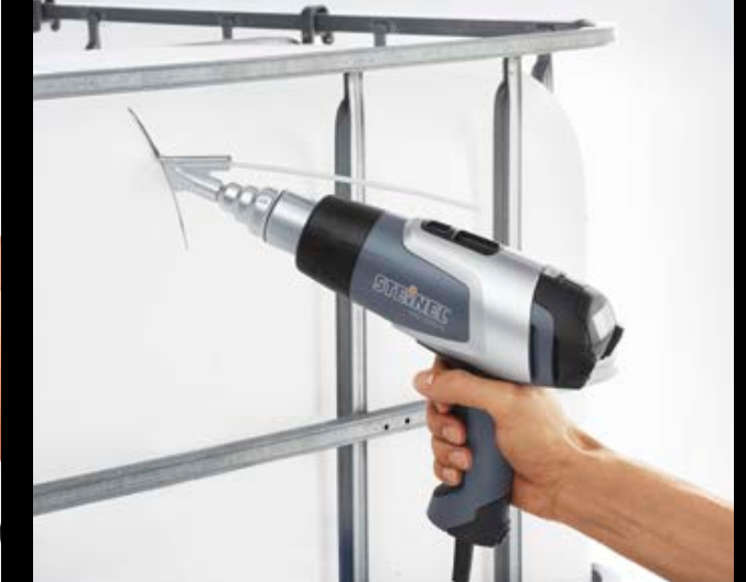
▲ Welding water tank HG 2320 E
