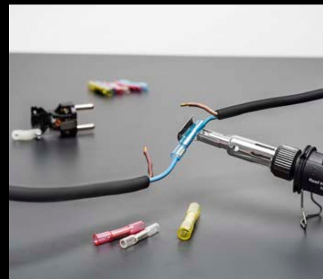
Create an even seal on solder sleeves
