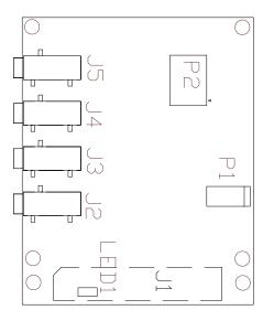
Figure 1-1. LED, Connector and Jumper Locations
