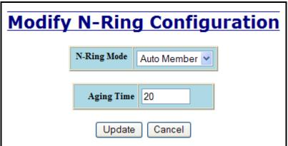
The N-Ring Aging Time has a default of 20 seconds and is separate from the Bridging Aging Time. N-Ring Aging Time is used when the switch is an N-Ring Manager or becomes an active N-Ring Member, and in either case N-Ring status includes for example:
