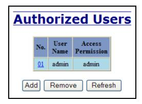
**Note:** There are a maximum number of 5 users per switch. User permissions have the right to view switch configurations and to view current port settings, but cannot make any changes to these settings. Admin permissions have the right to change and view any switch configuration and to change and view any current port settings.
