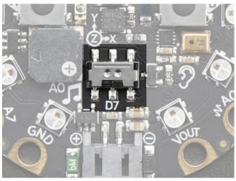
There is a single slide switch near the center bottom of the Circuit Playground Express. It is connected to digital #7. The switch is unconnected when slid to the left and connected to ground when slid to the right. Set pin #7 to use an internal pull-up resistor so that the switch will read HIGH when slid to the left and LOW when slid to the right.
