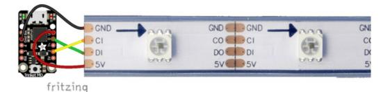
Note that the wire ordering on your DotStar strip or shape may not exactly match the diagram above. Check the markings to verify which pin is DIN, CIN, 5V and GND
