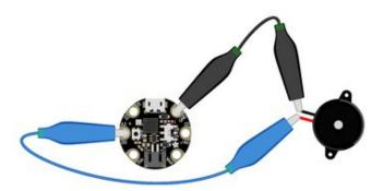
Use alligator clips to attach **A2** and **GND** to different legs on the piezo.
