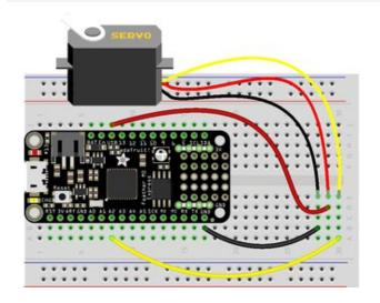
For boards like Feather M0 Express, ItsyBitsy M0 Express and Metro M0 Express, connect the ground wire to any GND, the power wire to USB or 5V, and the signal wire to A2.
