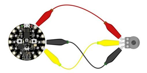
First, connect your potentiometer to the Circuit Playground Express using three alligator clip leads, as shown. The connections are:
