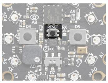
This small button in the center of the board is for **Resetting** the board. You can use this button to restart or reset the CPX.
