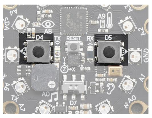
We're using the built-in pushbuttons in this example because it's very easy to get started, but you can use ALL KINDS of different buttons and switches, even homemade ones such as tinfoil or pennies, as digital inputs connected to the Digital IO pads!
