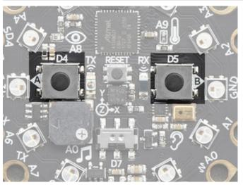
There are two large **A** and **B** buttons, connected to digital **#4** (Left) and **#5** (Right) each. These are unconnected when not pressed, and connected to 3.3V when pressed, so they read HIGH. Set the pins **#4** and **#5** to use an internal pull-down resistor when reading these pins so they will read LOW when not pressed.
