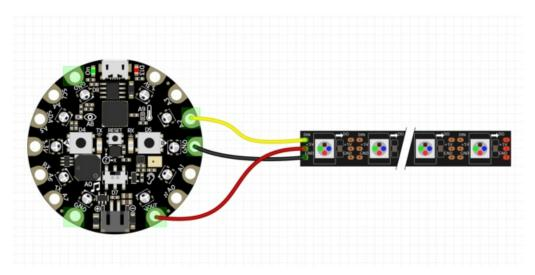
Verify the wiring on your strip or device - plugging into the 'DOUT' side is a common mistake! Wire up NeoPixels only while the Circuit Playground Express is not on, to avoid possible damage!
