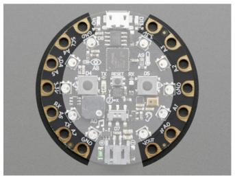
Of the 14 pads, you get a wide range of power pins, I2C, UART, Analog In, Digital In/Out, PWM, and Analog Out.
