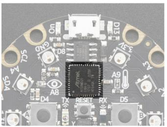
The **brains** of the operation here is the **ATSAMD21G18** a Cortex M0 microcontroller. This chip is much more powerful than the original Circuit Playground. It sits in the top center, and is what you use to run MakeCode, CircuitPython or Arduino!
