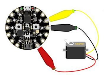
For Circuit Playground Express, use jumper wire alligator clips to connect the ground wire to GND, the power wire to VOUT, and the signal wire to A2.
