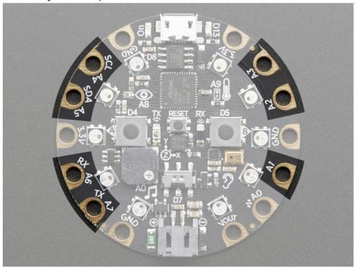
This quick-start example shows how you can read the capacitive touch sensors built into on seven of the Clrcuit Playground Express pads (pad **A0** is not a capacitive touch pad).
