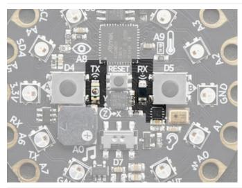
There's two elements for infrared. The **Transmitter** is on the left and is a big clear LED, this is connected via a transistor to pin #29
