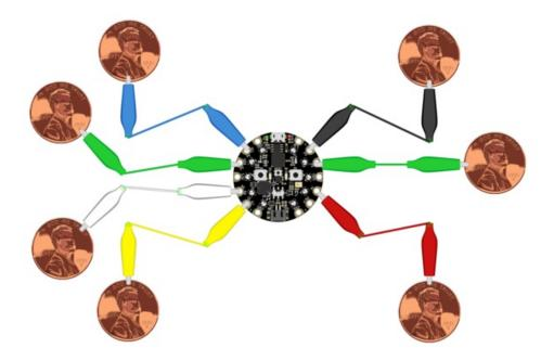
Capacitance is calibrated at startup, so you may need to reset the board after attaching leads to the pads
