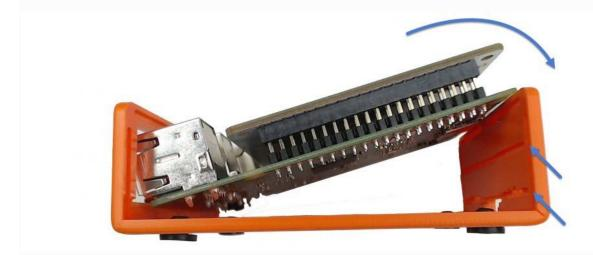
Once the two are fully rotated into position the Raspberry Pi and the Flick board should sit nicely in the bottom part of the case.
