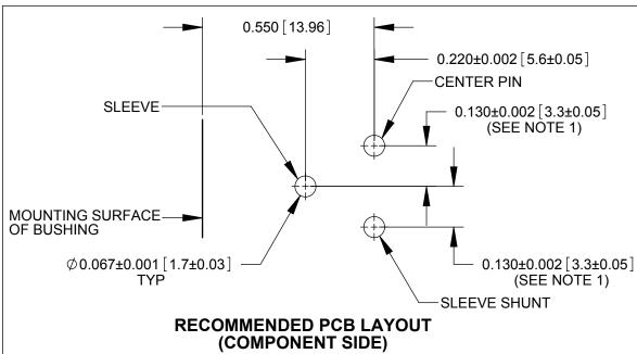
PART NUMBERDESCRIPTIONSWITCHCRAFT MATING 2.1mm POWER PLUGSL721RA2.1mm POWER JACK, LONG BUSHING, RIGHT-ANGLE PC767K, 768K
