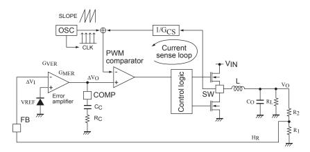
Fig. Current control loop of LV5768V
