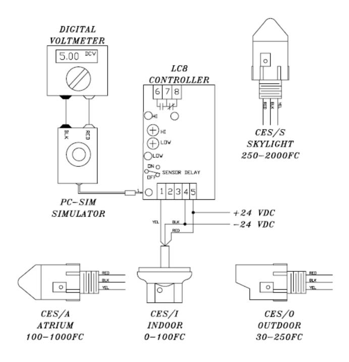
FIGURE 2: LC8 WITH CES SENSOR & PC SIMULATOR
