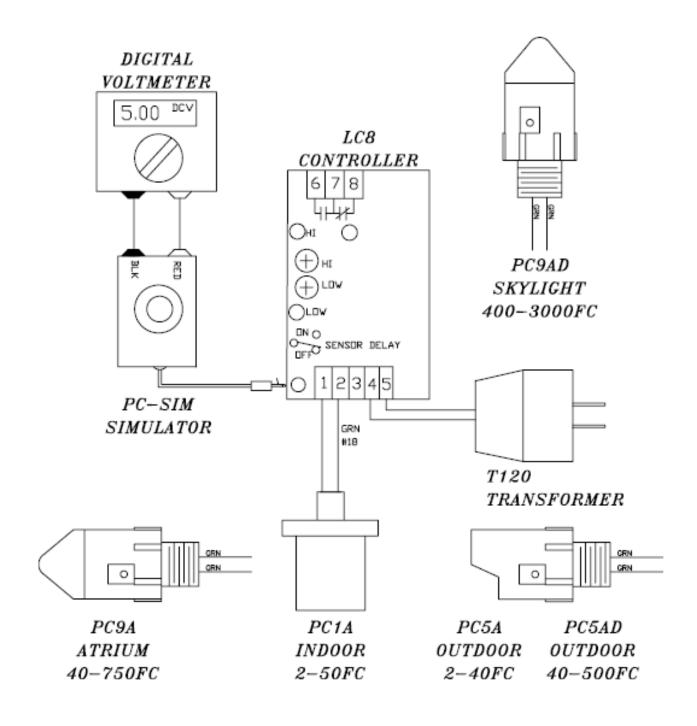
FIGURE 1: LC8 WITH PC SENSOR & PC SIMULATOR
