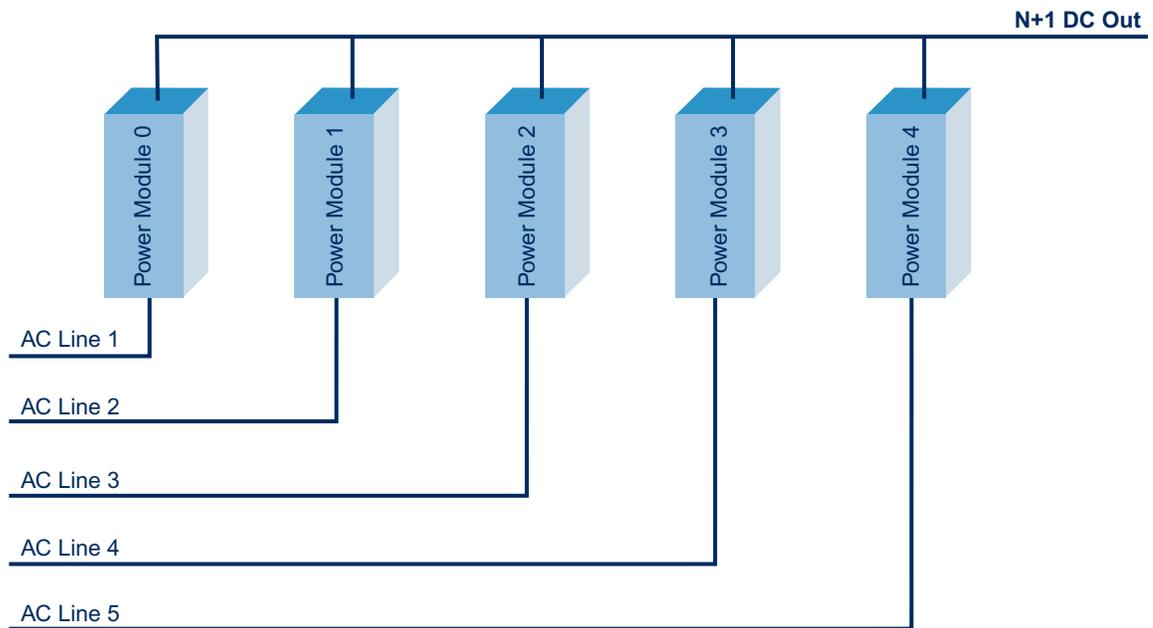
**Figure 3 - Individual Feed AC Wiring Architecture**
