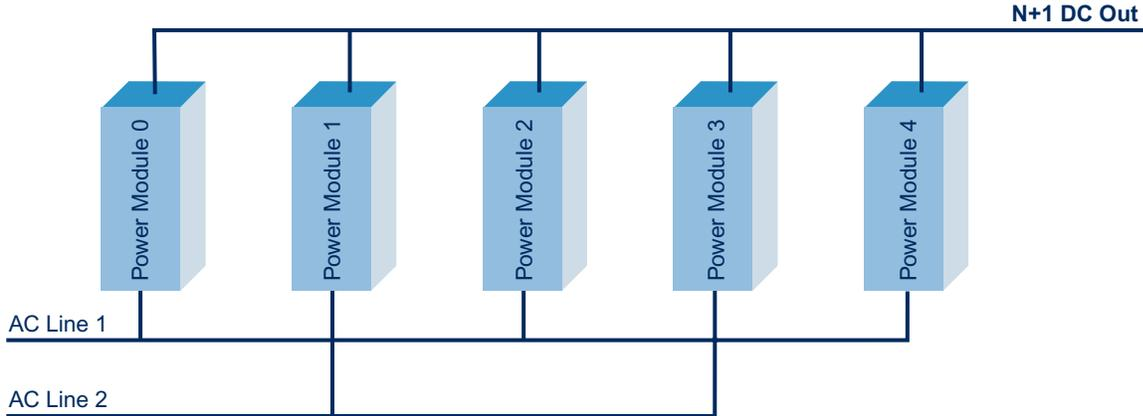
Figure 2 - Dual Feed AC Wiring Architecture
