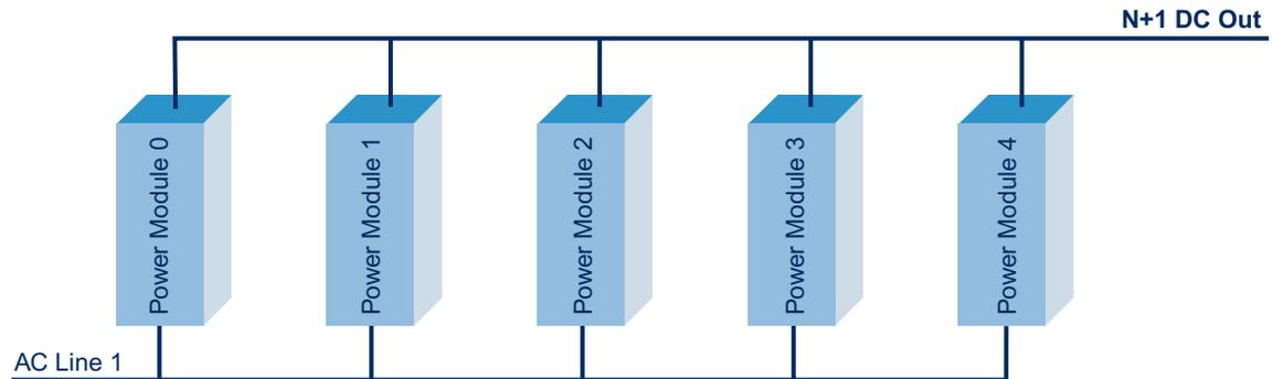
**Figure 1 - Single Feed AC Wiring Architecture**
