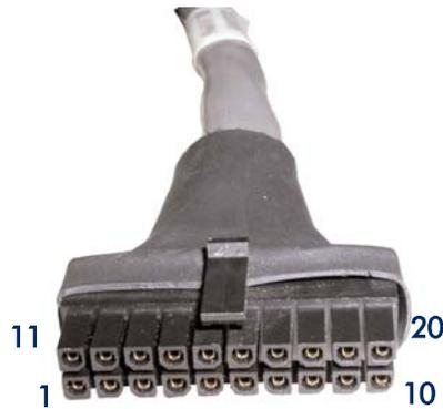
Figure 13 - Alarm cable pin out
