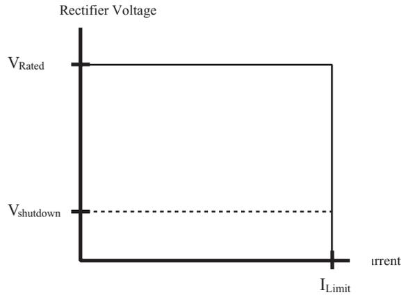
Figure 15 - Short Circuit & Current Limit
