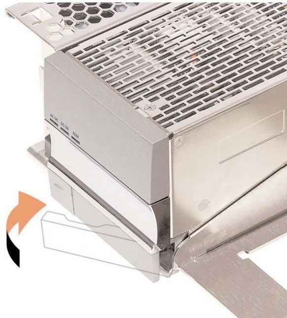
Figure 14 - Power module insertion
