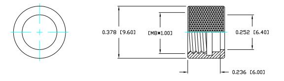
NΠΤF: MATERIAL HOUSING: PBT UL94V-0, BLACK CONTACT: PHOSPHOR BRONZE GROUND: BRASS SHELL: BRASS **D-RING**: **NBR FINISH** GOLD PLATED CONTACT: UNDER PLATE: NICKEL NICKEL 60 u BRIGHT TIN GROUND: SHELL: **NICKEL ELECTRICAL** RATED CURRENT: 5A 125V RATED VOLTAGE: INSULATOR RESISTANCE: 1000 MOhms MIN. CONTACT RESISTANCE: 10 mOhms MAX. IP67 WATER PROOF: **ENVIRONMENT** OPERATION TEMPERATURE: -40°C TD +85°C
