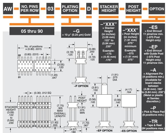
Note: For added mechanical stability, Samtec recommends mechanical board spacers be used in applications with gold or selective gold plated connectors. Contact jpg@samtec.com for more information
