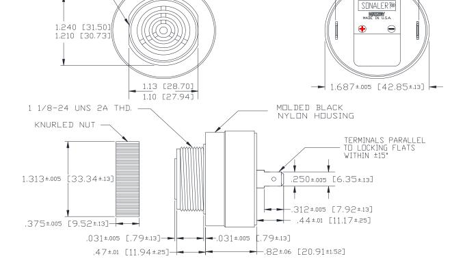
MOUNTING: REMOVE BLACK PLASTIC NUT AND INSERT THREADED FRONT THROUGH 1.25"
