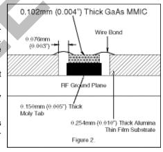
**General Handling:** Handle the chip along the edges with a vacuum collet or with a sharp pair of bent tweezers. The surface of the chip may have fragile air bridges and should not be touched with vacuum collet, tweezers, or fingers.
