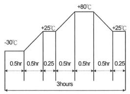
The diaphragm will be measured after being placed at +25°C for 4 hours. The value of the resonant frequency should be ±10%, the value of the electro static capacitance should be ±20% compared to the initial measurements. The resonant impedance should be 2,000  $\Omega$ max.
