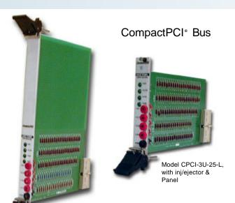
Resistive Load & Voltage Boards for 3U & 6U cPCI Applications
