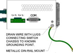
If the use of shielded cables is required, it is generally recommended to only connect the shield at one end to prevent ground loops and interfere with low level signals (i.e. thermocouples, RTD, etc.). Cat5e cables manufactured to EIA-568A or 568B specifications are required for use with N-Tron Switches.
