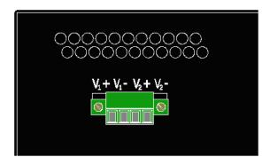
Unscrew & Remove the DC Voltage Input Plug from the top header.
