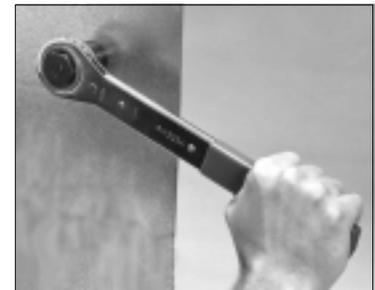
**4** Turn draw stud clockwise with the 34941 wrench until material is punched.
