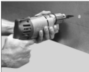
**1** The 1/2" conduit size punch requires 3/8" or larger pilot hole. Use Greenlee Kwik Stepper pilot step drills.
