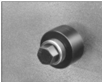
**6** For 3/4" through 2" conduit sized holes use 304AVBB 3/4" draw stud. Place selected size die on draw stud. Insert draw stud in 3/4" or larger pilot hole.\* Thread same size punch on the draw stud with the cutting edge toward the material being punched.
