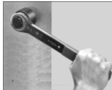
**7** Turn draw stud clockwise with 34941 wrench until material is punched.
