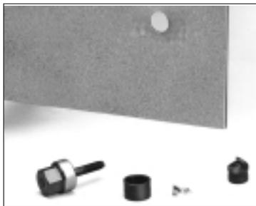
**5** Disassemble punch by turning draw stud counterclockwise while holding punch. Tip die and drop out split slugs.
