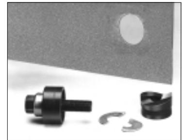
**8** Disassemble punch by turning draw stud counter-clockwise while holding punch. Tip die and drop out split slugs.
