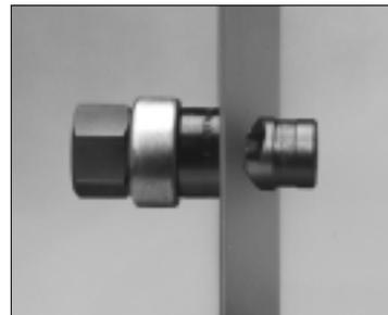
**3** Thread punch on draw stud with cutting edge toward material being punched.
