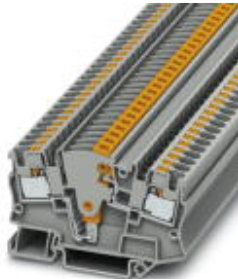
Test disconnect terminal block, Connection method: Push-in connection, Cross section: 0.2 mm 2 - 6 mm 2 , AWG: 24 - 10, Width: 6.2 mm, Color: white, Mounting type: NS 35/7.5, NS 35/15
