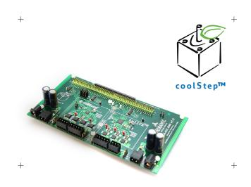
INFO The TRINAMIC TMCM-AC-840 Daughter Board Kit is an FPGA prototyping platform for power drivers for brushless DC motors (BLDC) as well as stepper motors. The TMCM-AC-840 Daughter Board Kit incorporates one TMC603A BLDC motor driver IC and one TMC262 coolStep<sup>™</sup> stepper motor driver IC as well as two fitting motors to start prototyping right away.
