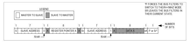
Figure 6. Reading from a single register.
