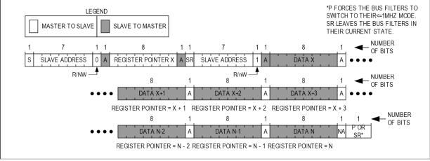
Figure 7. Reading from multiple registers.
