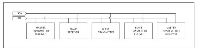
Figure 2.  $I^2C$  system configuration.
