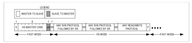
Figure 8. Engaging high-speed mode.
