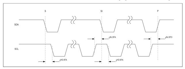
Figure 3. I<sup>2</sup>C START and STOP conditions.
