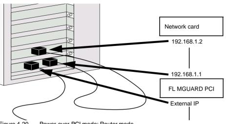
Figure 4-20 Power-over-PCI mode: Router mode
