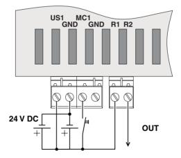
Figure 3-6 Supplying the device using two voltage sources
