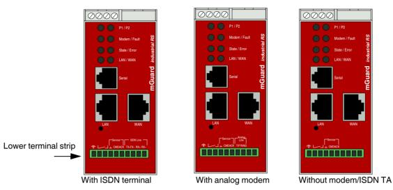
Figure 4-2 FL MGUARD RS ...: Lower terminal strip
