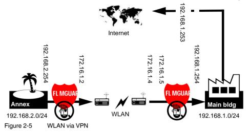
In this example, the FL MGUARD devices were set to *router* mode and a separate network with 172.16.1.x addresses was set up for the WLAN.
