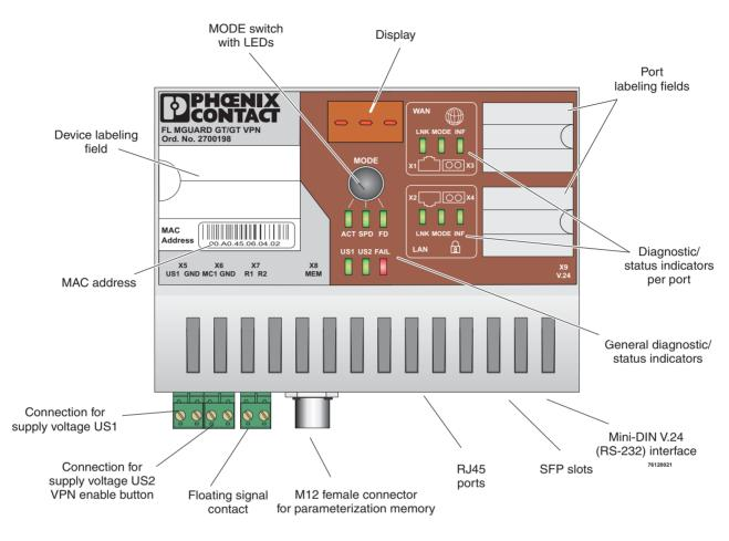
Figure 3-2 Operating elements and indicators on the FL MGUARD GT/GT ...
