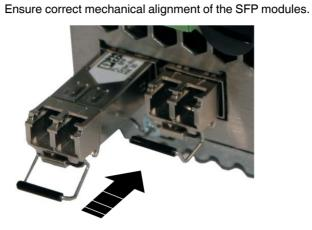
Figure 3-8 Inserting the SFP modules
