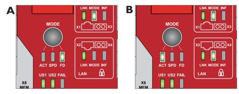
Figure 3-13 Example for status indicators on the FL MGUARD GT/GT ...
