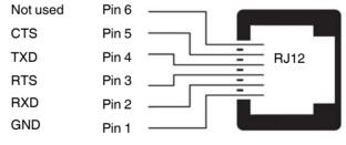
Figure 4-6 Pin assignment of the RJ12 female connector (serial port)
