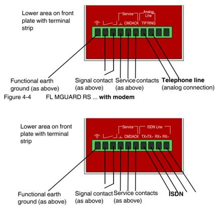
Figure 4-5 FL MGUARD RS ... with ISDN terminal adapter
