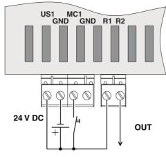
Figure 3-5 Supplying the device and connecting the VPN enable button using one voltage source
