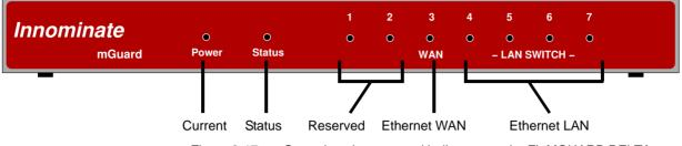
Figure 3-17 Operating elements and indicators on the FL MGUARD DELTA
