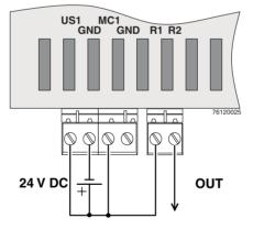
Figure 4-8 Simple connection of the supply voltage/signal contact without VPN enable button
