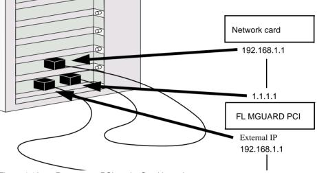
Figure 4-19 Power-over-PCI mode: Stealth mode
