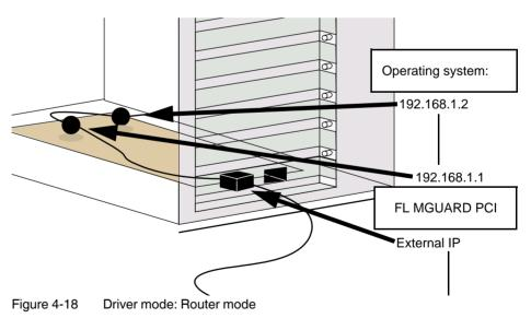
If the FL MGUARD is in *router* mode (or *PPPoE* or *PPTP* mode), it essentially creates its own network with the operating system of the computer in which the FL MGUARD is installed.
