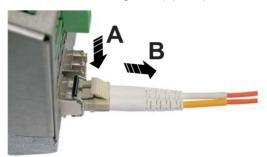
Figure 3-9 Removing the fiber optic connectors
