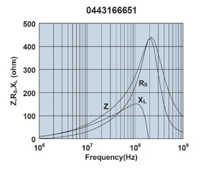
Impedance, reactance, and resistance vs. frequency.
