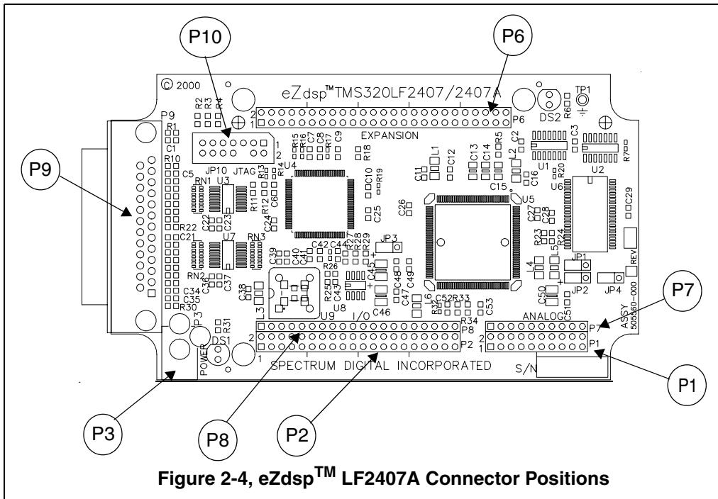
**Figure 2-4, eZdsp™ LF2407A Connector Positions**
