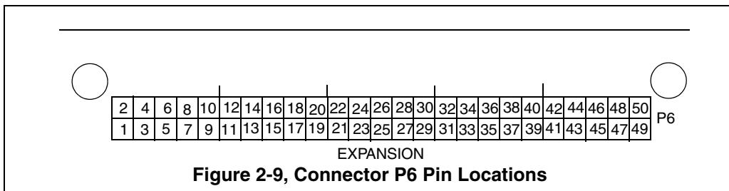
The definition of P6, which has the memory interface signals, is shown below.
