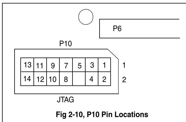
The definition of P10, which has the JTAG signals is shown below..
