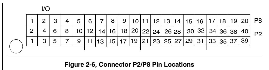
The definition of P2, which has I/O signal interface is shown below.
