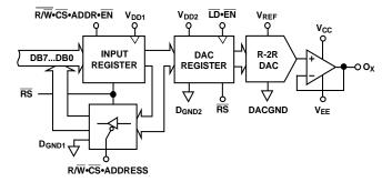
Figure 1. Equivalent DAC Channel
