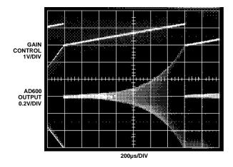
Figure 24. Time Dependent Gain of the AD600
