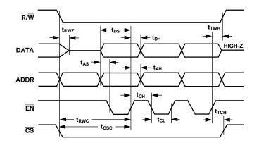
Figure 2. Write Timing
