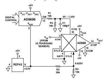
Figure 23. Ultrasound Amplifier with Digitally Controlled Variable Gain
