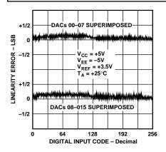
Figure 5. Linearity Error vs. Digital Code
