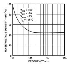
Figure 10. Voltage Noise Density vs. Frequency
