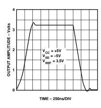
Figure 9. Full-Scale Settling Time
