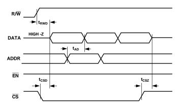
Figure 3. Readback Timing
