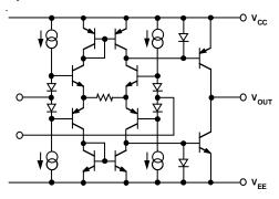
Figure 17. Equivalent Analog Output Circuit
