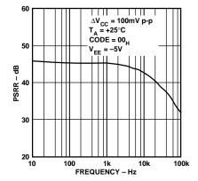
Figure 13. PSRR vs. Frequency
