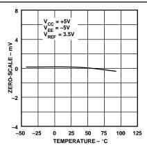
Figure 7. Zero-Scale Voltage vs. Temperature
