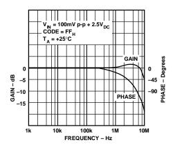
Figure 11. Gain & Phase vs. Frequency
