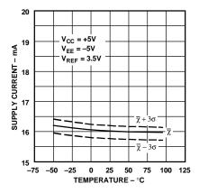
Figure 14. Supply Current vs. Temperature
