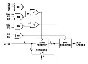
Figure 19. Logic Interface Circuit for DAC Channel 0
