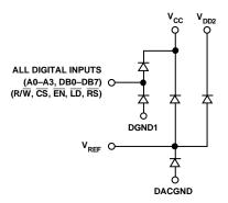
Figure 18. ESD Protection Diode Locations
