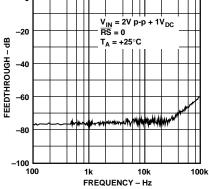
Figure 12. AC Feedthrough vs. Frequency
