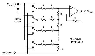
Figure 16. Equivalent Schematic of Analog Channel voltage. The switches' low ON resistance and matching is important in maintaining the accuracy of the R-2R ladder.
