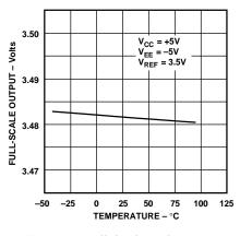
Figure 6. Full-Scale Voltage vs. Temperature
