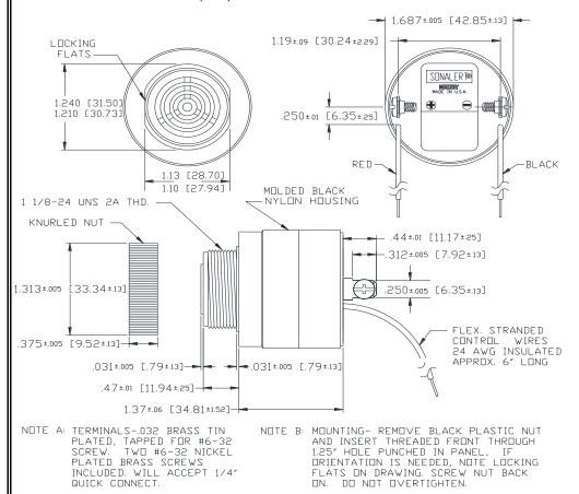
The red and black leads control the several functions. A logic 'Low' is a voltage less than 1/3 of supply voltage. A logic 'High' is a voltage greater than 1/2 supply voltage. A red or black input lead left unconnected is considered an open state.
